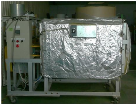
Prototype 3 firing furnace reproduced in 2015
